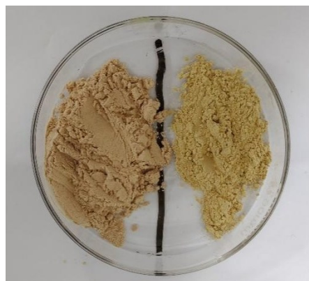
图1 未改性玉米芯粉(左)与改性玉米芯粉(右) Fig.1 Unmodified corn cob powder (left) and modified corn cob powder (right)
